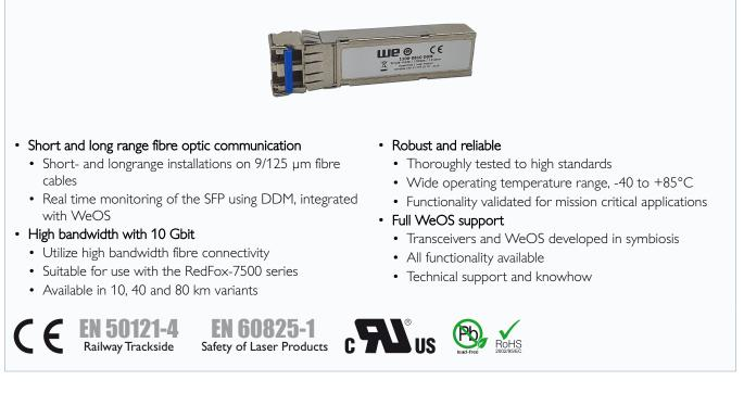
10 Gbit Singlemode SFPs are suitable for short- and longrange applications requiring high bandwidth. The available models can use singlemode fibre cables with a core of 9 µm. Using the DDM functionality, which is fully integrated into WeOS, it is possible to monitor parameters such as temperature, TX/RX power and voltage, ensuring correct operation.
