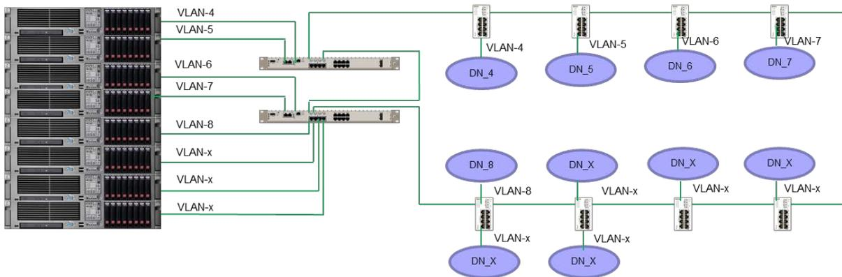
Each DN\_x is a different protocol running in a VLAN
